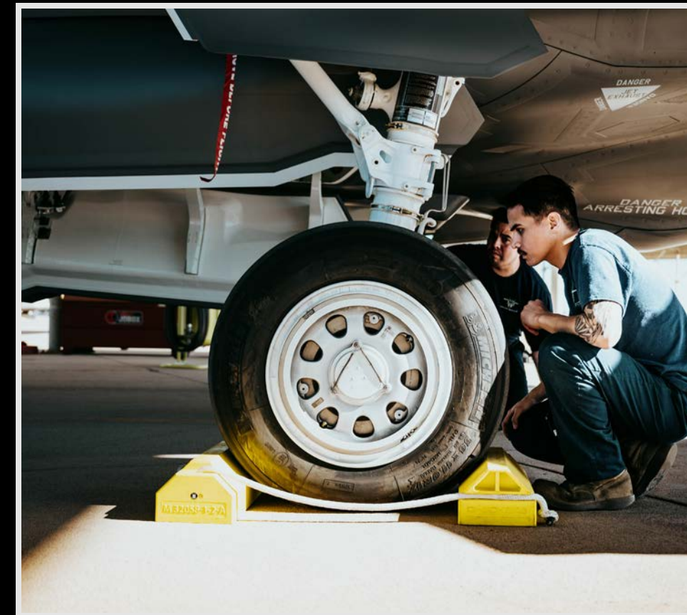
Left: Maintenance personnel carries out post-flight checks on the aircraft while the pilot prepares to exit the cockpit Above: Two maintenance technicians check the left main landing gear for tire and brake wear.
