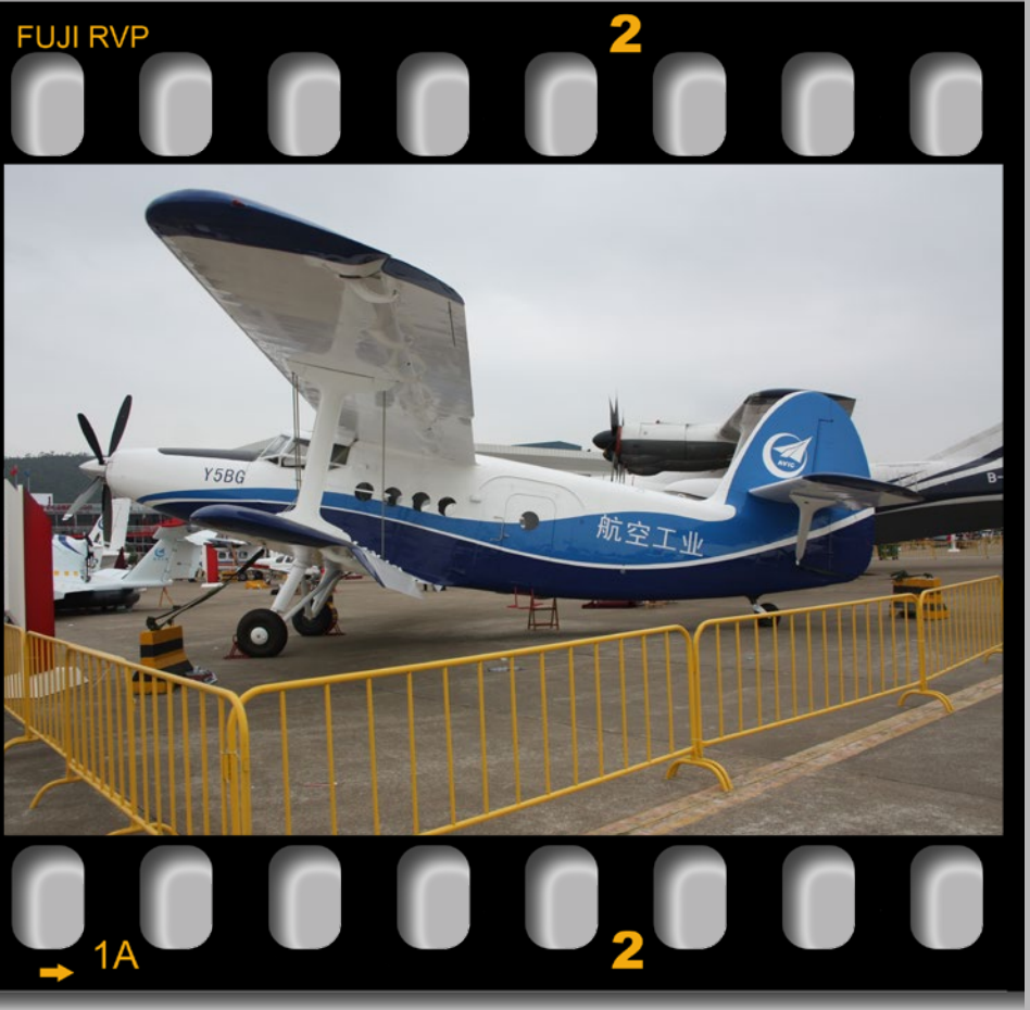
The AVIC Y5B6 is a Chinese licence built Antonov An-2. This particular aircraft is equipped with a Honeywell TPE331-UAN turbo-prop engine (above)
