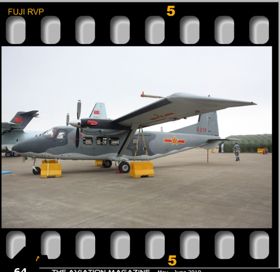
The AVIC Y5B6 is a Chinese licence built Antonov An-2. This particular aircraft is equipped with a Honeywell TPE331-UAN turbo-prop engine (above)
