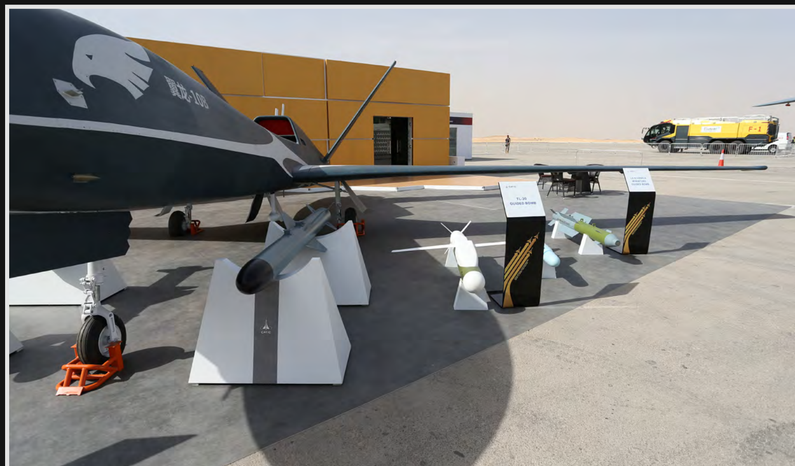
The Wing Loong-10 drone – military designation WZ-10 is a High-Altitude Long Endurance (HALE) UAV, featuring some stealth characteristics. In 2017, it was developed by the Chengdu Aircraft Industry Group for reconnaissance and precision strike missions
