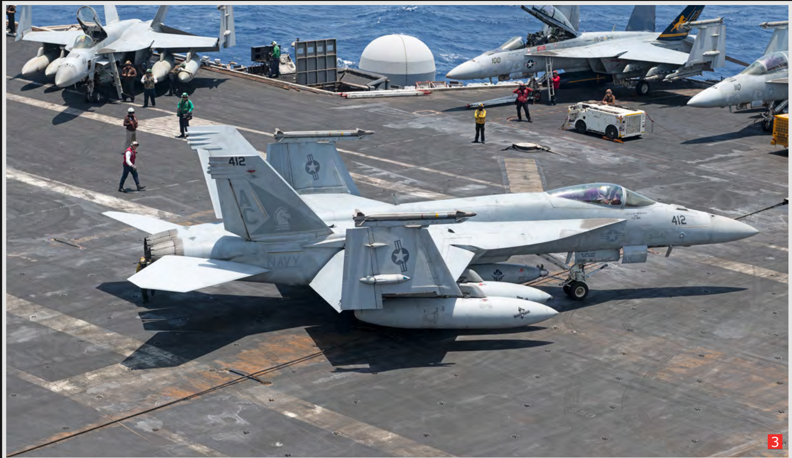
The F/A-18E Super Hornet (VFA-105) can fold its wings to reduce the space needed when the aircraft is parked. This is typical for carrier-based aircraft
